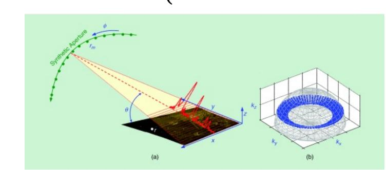
With active electronically steerable arrays (AESA), we can simultaneously image multiple scenes via sub-Nyquist sampling.
