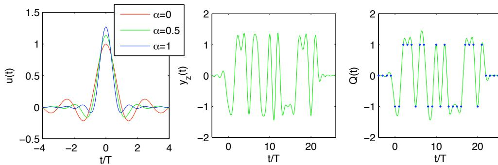
In practice, the pulse would be shifted forward  $T_u/2$  seconds and then restricted to the interval  $t \in [0, T_u]$ .
