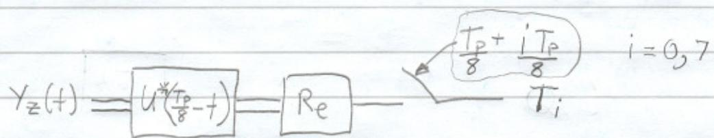
$$T_i = \operatorname{Re} \left[ \int_{\frac{iT_p}{8}}^{\frac{(i+1)T_p}{8}} Y_z(t) dt \right] \Rightarrow \text{only one filter sampled 8 times}$$
