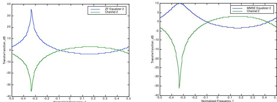
Note noise amplification of ZF equalizer! Results in an SNR loss of about 17 dB relative to the flat channel case.
