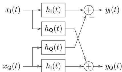
Passband additive white Gaussian noise model [Ch. 3]:
