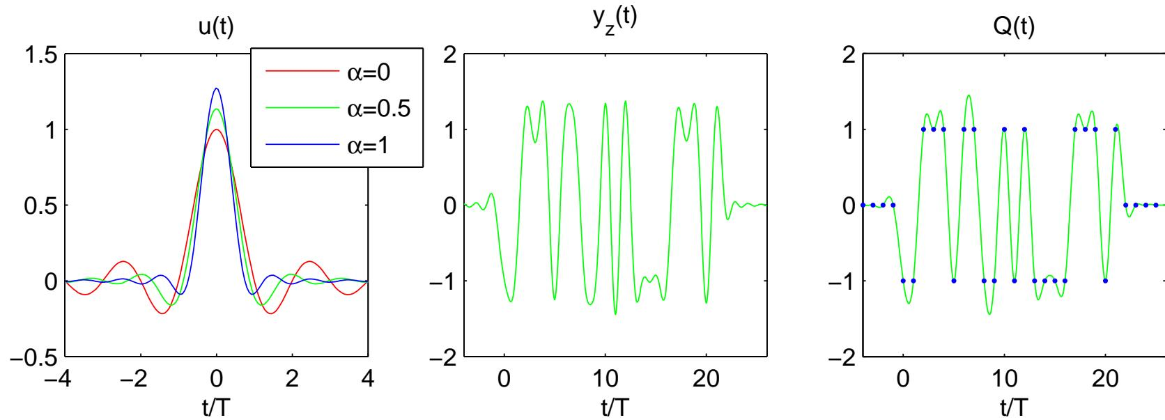
Note: non-causal (for simplicity). To make causal, shift pulse forward  $T_u/2$  seconds and set to zero for  $t \notin [0, T_u]$ .
