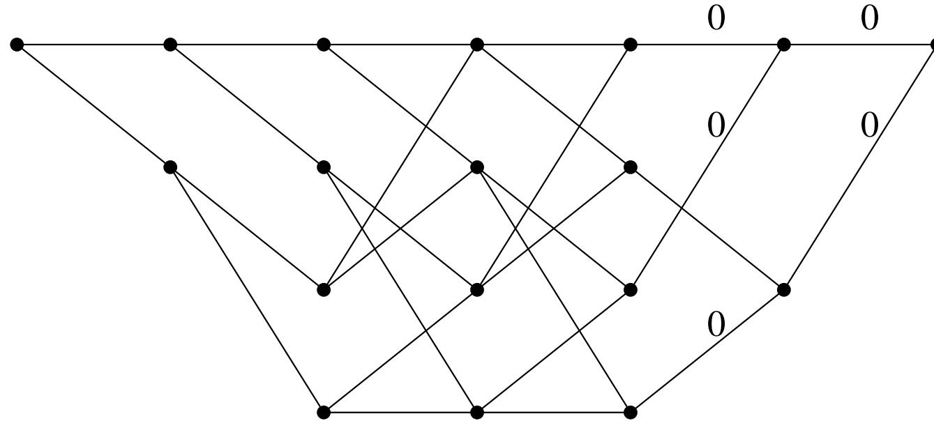
Here,  $\nu_c = 2$  additional zero-bits are used to return to initial state (“termination”). Thus, for  $R = 1$ , have frame length  $N_f = K_b + \nu_c$ . Note  $R_{\text{eff}} = \frac{K_b}{K_b + \nu_c} \approx 1 = R$  for large  $K_b$ .
