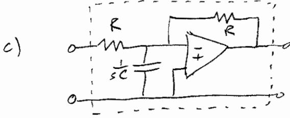
Realizing that the input terminals are at the same voltage
