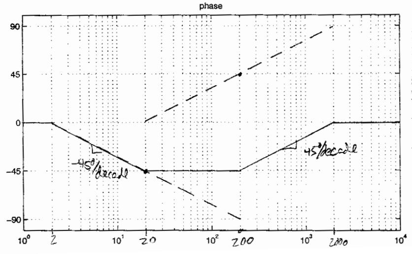
4) These were a few designs that implemented  $-\frac{1}{10} \cdot \frac{s+10}{s+1}$  using a single op-amp, no inductors, and 1μF capacitors.
