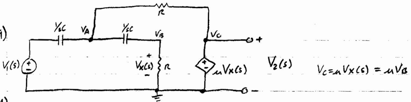
$$\text{Node A: } (Cs + 1/R + Cs)VA - CsVB - \frac{\mu V_B}{R} = CsV_1(s)$$
